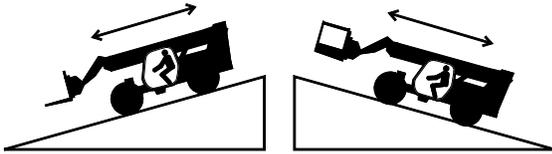
On steep terrain, drive only up and down hill, and always keep the machine in gear. Do not turn across slope when machine is traveling up or down a slope. To avoid overspeeding the engine and transmission when driving down slopes, downshift to a lower gear and use the service brake as necessary to maintain a slow speed.
