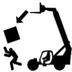
Do not raise a load unless the load is properly positioned or secured on the forks or approved attachment.
