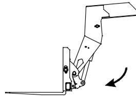
Tilt the forks back to pivot the quick attach into the attachment.
