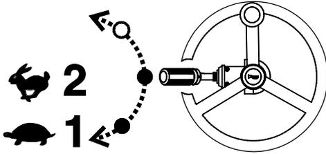
Come to a complete stop before shifting the transmission from forward to reverse. The transmission control lever must be in 1st or 2nd gear only.
