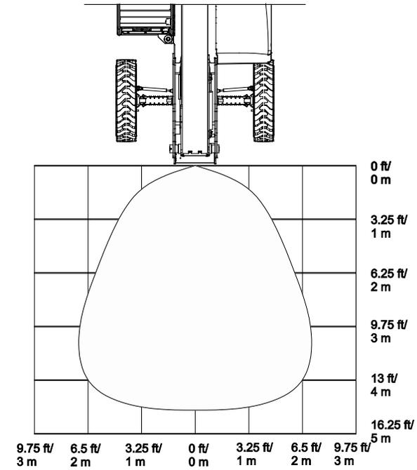
Approximate detection range. Minimum rear proximity sensor detection height is 2 ft/0.6 m.
