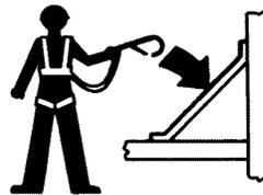
Occupants must wear a safety belt or harness in accordance with governmental regulations. Attach the lanyard to the anchor provided in the platform.
