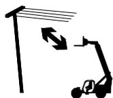
Always contact the electrical power line owner. The electrical power shall be disconnected or the power lines moved or insulated before machine operations begin.
