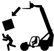
Keep people, equipment and material out of the work area. Do not operate the machine while people are under or near an elevated boom, whether it is loaded or unloaded.
