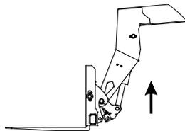
Raise the boom until the pin is secured in the hooks on the attachment.
