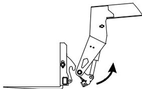
Tilt the forks forward to pivot the quick attach connector back.
