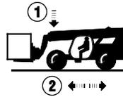
When driving, keep the boom at or below horizontal and keep the load close to the ground.
