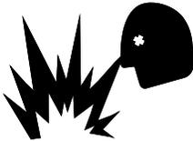
Keep sparks, flames, and lighted tobacco away from batteries. Batteries emit explosive gas.
